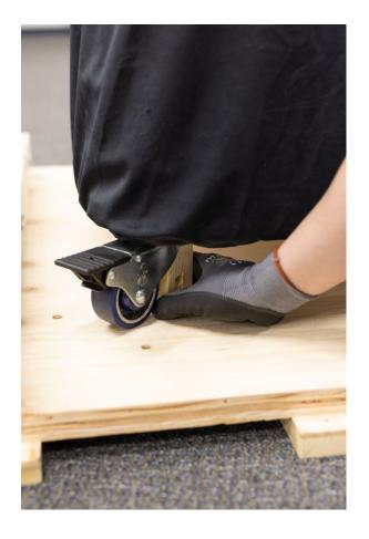
8. Apply the ramp the front of the crate base, hooking in the locator pins to secure. Turn the front casters to be positioned under the speaker. Roll the speaker down the ramp carefully.
