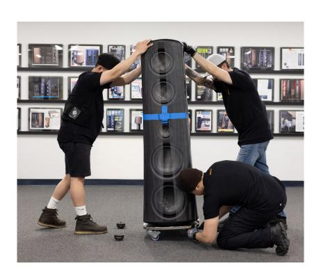
12. Repeat the last step by tilting the speaker in the opposite direction, onto the MPods. Remove the casters, apply the remaining two MPods and return gently to the floor.
