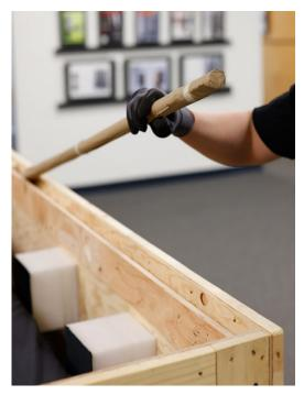
3. Locate the ramp inside of the crate. Lift it up and away from the crate
