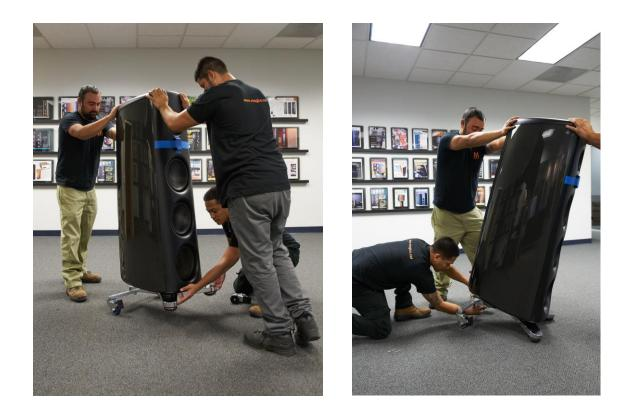
**15.** TILT SPEAKER FORWARD, UNTHREAD AND REMOVE THE SHIPPING BARS FROM THE BOTTOM OF THE M6. YOU WILL NEED A 3/8" HEX BIT TO REMOVE THE LARGE FASTENER ON THE SHIPPING BAR.
