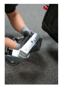
**17.** CAREFULLY THREAD THE M-POD INTO THE REAR OF THE M2 BASE AND LOWER THE M2 ON TO ALL 3 M-PODS
